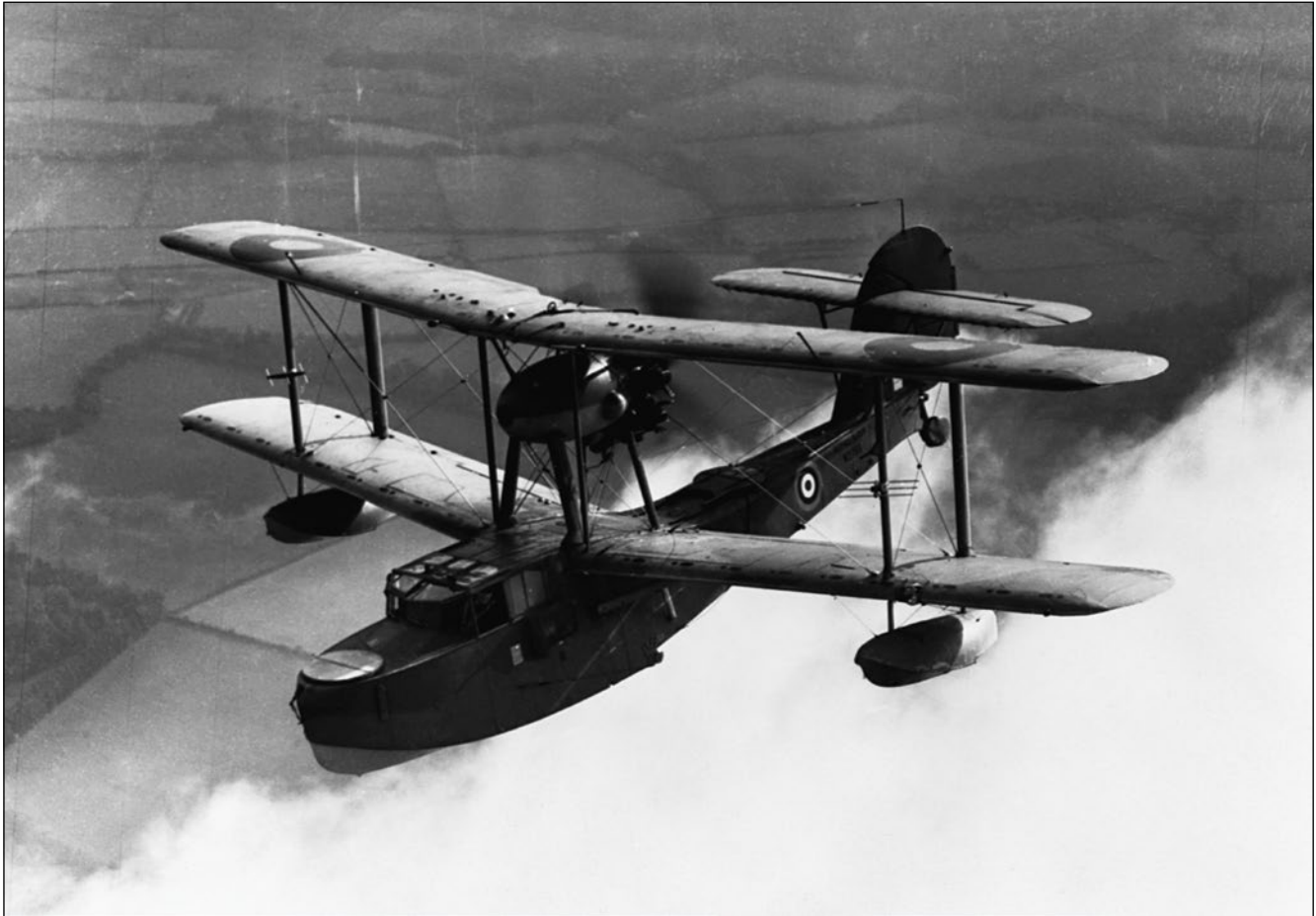
A Supermarine Walrus air/sea rescue aircraft used to recover downed airmen during the Second World War
